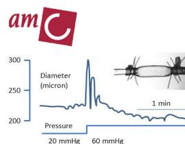
A single artery, maintained alive and mounted between two glass pipettes that allow pressurization and perfusion. A step increase in pressure causes mechanical distension followed by downregulation of the diameter due to the smooth muscle cells within a minute.
