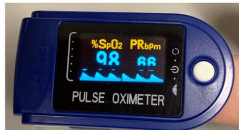
*Based on the ratio of two wavelengths and clever algorithm, the arterial oxygen level can be measured with a simple device.*
